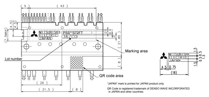
Fig.2-3-2 Laser marking view PSSxxS72FT (Dimension in mm)
