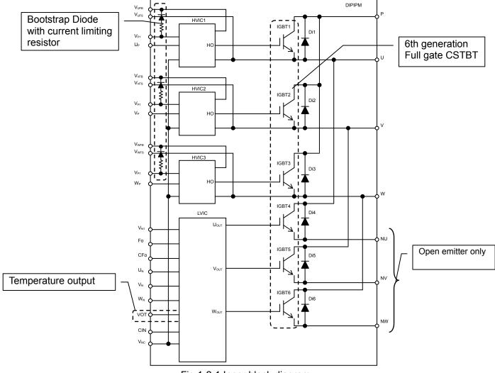
Fig.1-2-1 Inner block diagram
