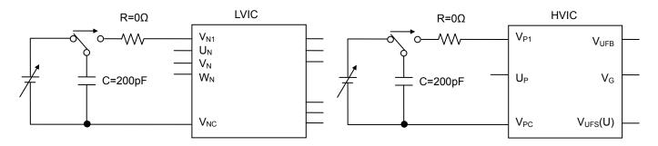
Fig.3-3-3 LVIC terminal Surge Test circuit
