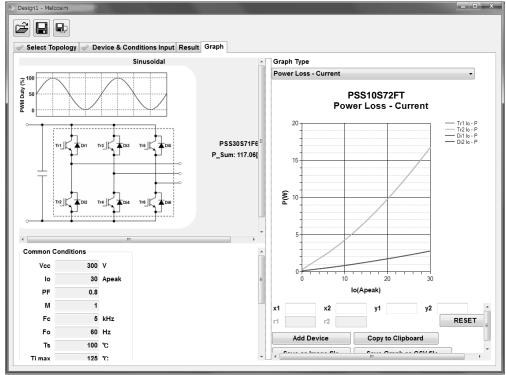
Fig.3-2-3 Loss simulator screen image
