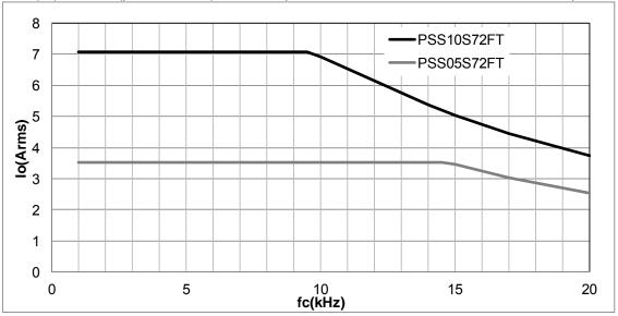
Fig.3-2-2 Effective current-carrier frequency characteristics
