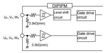
Fig.3-1-5 Internal structure of control input terminals
