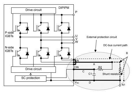
Fig.3-1-12 External protection circuit
