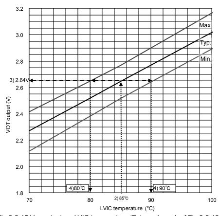
Fig.2-2-15 V<sub>OT</sub> output vs. LVIC temperature (Enlarged graph of Fig.2-2-12)
