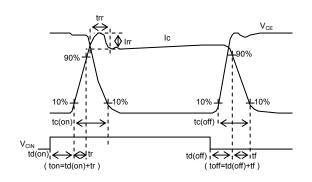
Fig.2-1-4 Switching time definition
