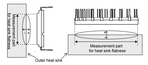
Fig.2-4-2 Measurement point of heat sink flatness(PSSxxS71F6)
