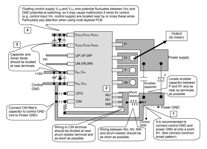
Fig.3-1-13 Precaution for wiring on PCB
