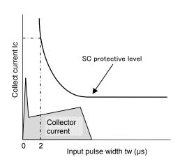
Fig.2-2-2 Filter time constant setting
