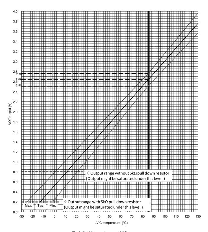
Fig.2-2-12 V<sub>OT</sub> output vs. LVIC temperature
