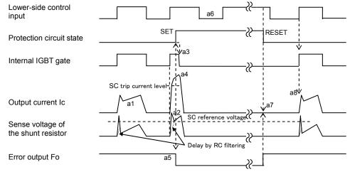
Fig.2-2-3 SC protection timing chart
