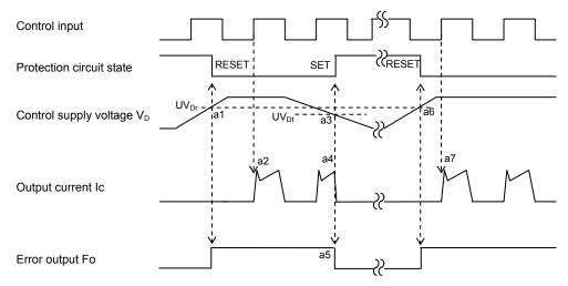
Fig.2-2-4 Timing chart of N-side UV protection
