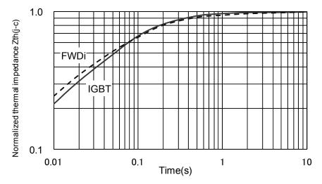
Fig.2-1-3 Typical transient thermal impedance (PSSxxS72FT)
