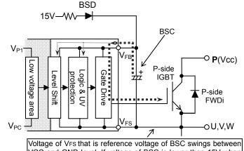
Voltage of VFs that is reference voltage of BSC swings between VCC and GND level. If voltage of BSC is lower than 15V when VFs becomes to GND potential, BSC is charged from 15V N-side control supply.
