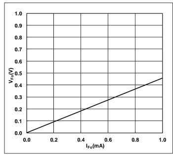
Fig.3-1-8 Fo terminal typical V-I characteristics (V<sub>D</sub>=15V, T<sub>i</sub>=25°C)
