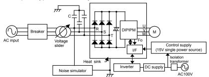
Fig.3-3-1 Noise withstand capability evaluation circuit
