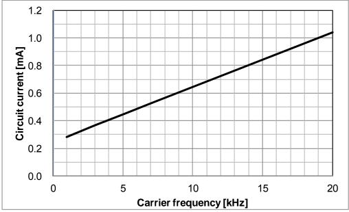
Fig.4-2-1 IDB vs. Carrier frequency for PSS05S72FT
