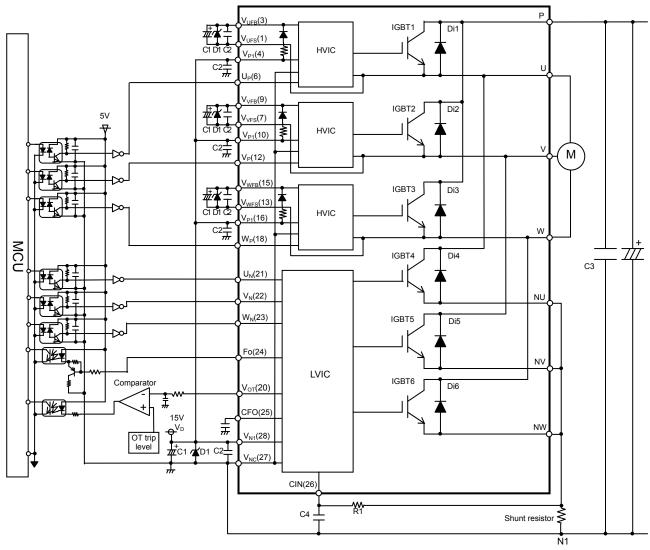
Fig.3-1-3 Interface circuit example with opto-coupler
