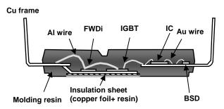
Fig.1-1-2 Internal cross-section structure
