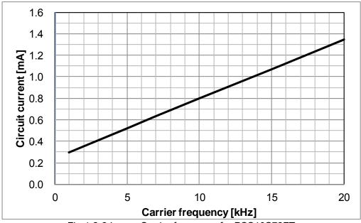
Fig.4-2-2 I<sub>DB</sub> vs. Carrier frequency for PSS10S72FT
