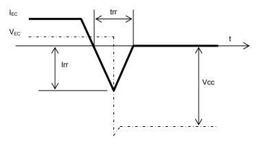
Fig.3-2-1 Ideal FWDi recovery characteristics curve
