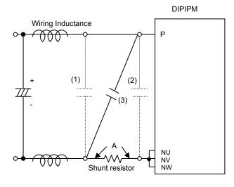
Fig.3-1-9 Recommended snubber circuit location
