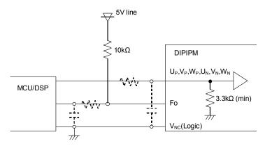
Fig.3-1-6 Control input connection
