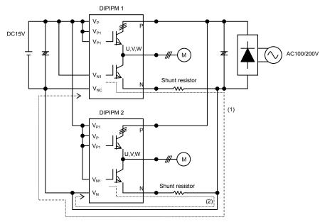
Fig.3-1-14 Parallel operation
