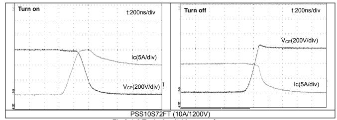
Fig.2-1-6 Typical switching waveform
