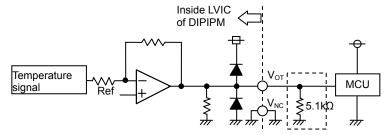
Fig.2-2-9 V<sub>OT</sub> output circuit in the case of detecting low temperature
