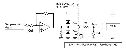
Fig.2-2-11 V<sub>OT</sub> output circuit in the case with high protection level
