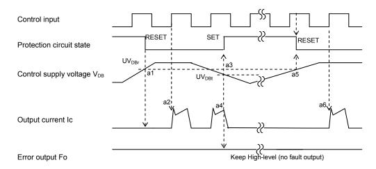
Fig.2-2-5 Timing Chart of P-side UV protection
