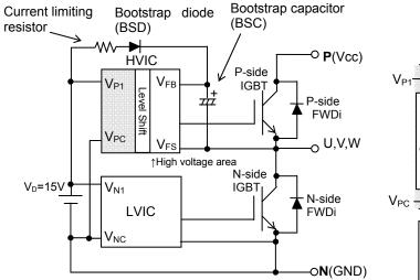
Fig.4-1-1 Bootstrap Circuit Diagram
