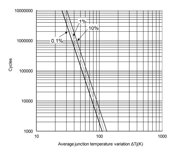
Fig.3-1-18 Power cycle curve
