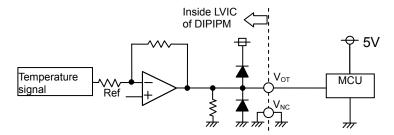
Fig.2-2-8 V<sub>OT</sub> output circuit
