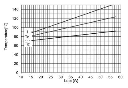
Fig.2-2-13 Example of relationship of Tj, Tc, Tic (One IGBT chip turns on. DC current Ta=25°C)
