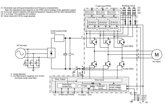
Fig.3-1-1 System block diagram (Example)
