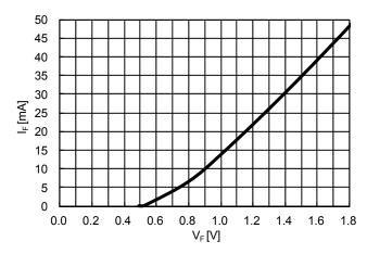
Fig.4-3-1 V<sub>F</sub>-I<sub>F</sub> curve for bootstrap Diode (The right figure is enlarged view)
