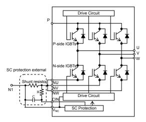
Fig.2-2-1 SC protecting circuit
