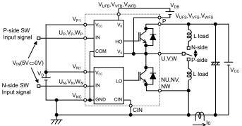
Fig.2-1-5 Evaluation circuit (inductive load)
